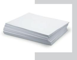
**Wood-free papers,** also known as chemical pulp or free sheet papers, are specially manufactured types of paper without groundwood pulp. They primarily contain cellulose fibers derived from chemically treated plant matter, mainly bleached kraft pulp obtained from coniferous trees or recycled fibers. The absence of groundwood results in improved brightness, opacity, cleanliness, and higher archival permanence compared to conventional papers containing groundwood.
